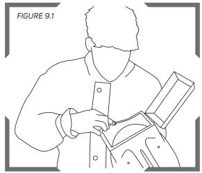
Make sure the inner lens gasket seal is securely fitted in the helmet with no cracks or tears in the seal. Check that the inner lens is correctly fitted into the gasket.
