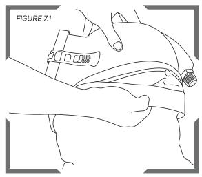
First remove the cape cover band to reveal the eight snaps. The cape can then easily be removed by undoing the snaps.
