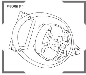
Having removed the cape, wipe out the inside of the helmet with a soft cloth and mild detergent or a disinfectant wipe. Check the inside for cracks in the shell, damage to the air inlet and head harness.
